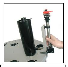
(4) Fit this assembly to the turntable. Canister screws (already fitted to the canister) fit into the inner ring location keyholes and the remote bracket fits into the 4 slots simultaneously. Push firmly into position. If the bracket face is not firm against the turntable edge, then the extension tube is not correctly fitted.
