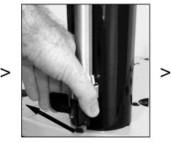
Release the valve lever slowly and the drop will withdraw into the nozzle
