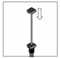
(1) After lightly oiling the top inside edge of the cylinder, position the plunger assembly on the cylinder with one hand. With the palm of the other hand, firmly push the plunger down fully.
