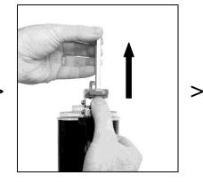
With the appropriate button operated, lift the gauge to the reading required.
