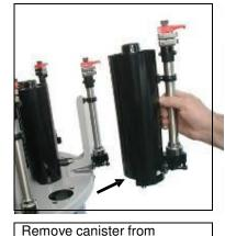
Remove canister from turntable and drain colorant into a clean container
