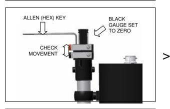
(3) Carefully wind one grubscrew down until only slight movement is felt between the outer pump handle and the gauge knob. Then wind the other grubscrew down until no free movement can be felt, being careful not to over-adjust.
