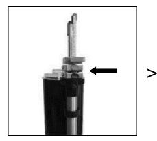
According to the setting required, operate the spring loaded button to release the gauge. The red knob is for the red gauge and the black knob is for the black gauge
