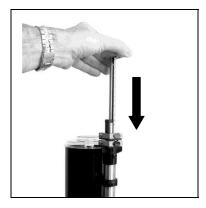
Push the pump handle down fully to dispense colorant into the cup
