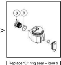
Reassemble and refit canister to turntable
