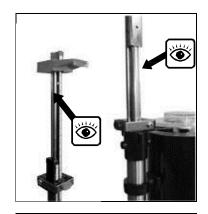
Raise the pump handle to its maximum extension and examine the pump shafts for signs of colorant. This indicates that the piston seal will need replacement (see Chapter VI - E,F,G)
