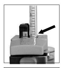
The correct gauge setting is shown when the figure selected is fully exposed above the RED handle and the gauge release button clicks firmly into place.
