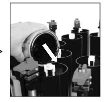
Pour the contents of each colorant can into the correct canister. Discard the colorant can and replace the canister lid
