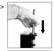
Discharge the colorant back into the canister by depressing the pump handle fully. Repeat this process 30 times.
