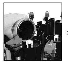
Check the level of colorant and top up if required
