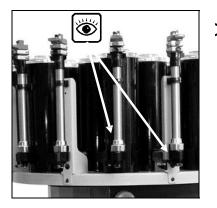
Inspect the function of the valve and the canister for leaks
