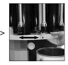
Rotate the turntable so that the pump of the appropriate canister is directly over the can. If the detent lever is released it will lock the canister into the correct position. You may need to move the turntable slightly from side to side to allow the locking pin to locate the locking hole.
