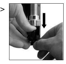
If dried colorant is found to be blocking the nozzle, open the valve to remove and replace the nozzle. Ensure the o-ring is retained. Clean the nozzle using warm soapy water
