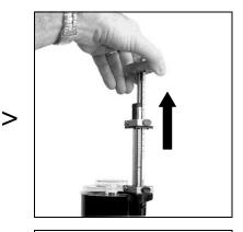
Without operating the valve lever lift the pump handle to its maximum travel (this draws the colorant into the canister)
