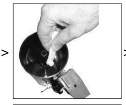
If required, tighten or replace valve insert sleeve (with the wrench supplied). Take care not to over tighten or sleeve with crack.
