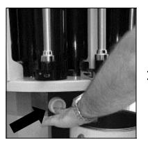
Depress and hold the detent lever to release the turntable. You can lock the detent lever in the release position by pushing it sideways.
