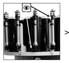
Examine the machine for loose canisters and loose cylinder caps. Tighten if necessary
