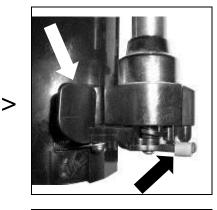
Check the valve levers and nozzle wiper arms for possible damage.
