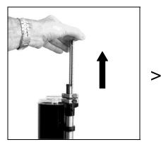
Lift the pump handle to its maximum travel
