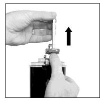
Set the gauge or gauges of each pump to its halfway point by operating the spring loaded button then lifting the gauge by its handle
