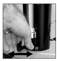
Open and close each pump valve 5 times
