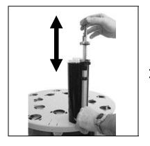
Purge the pumps (see chapter IV, step 2 & 3) however only operate the pump 5 times
