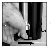
Open the valve lever **without operating the pump.** A small drop of colorant will appear at the nozzle
