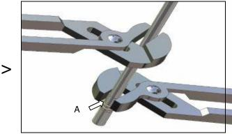
(2) Using two pairs of pliers, grip the inner end of the piston (A) with one and the piston shaft with the other. Unscrew the piston (using a little heat if difficult) and discard.
