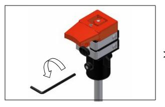
(1) Loosen both grubscrews in the cylinder of the end cap (use Allen key provided) and remove the plunger assembly from the cylinder. Remove the gauges from the plunger assembly, then withdraw the inner plunger assembly from the hollow outer plunger shaft. Clean all colourant from both plunger assemblies.
