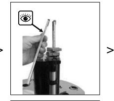
Examine gauges for damaged graduated scales or worn holes and replace if necessary
