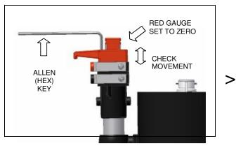
(5) Using the Allen key, undo the calibration grubscrew in the red pump handle until free movement can be felt in the handle. Carefully wind the grubscrew back down until no free movement can be felt between the red pump handle and the red gauge knob. **Be careful not to over-adjust.**
