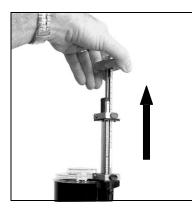
With the gauges correctly set, slowly and gently lift the red pump handle until both red and black handles are against the appropriate gauge knobs
