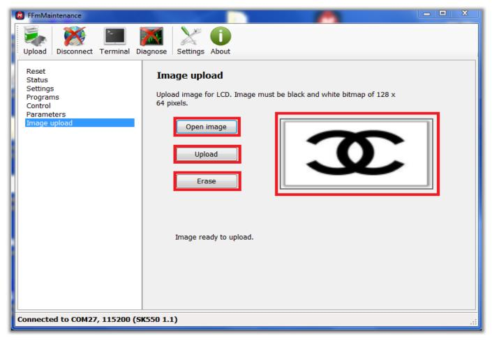
This feature allows the user to select and upload a chosen image to the machine. This feature only works in combination with firmware version 3.16 The image  $\underline{must}$  be a black and white bitmap-picture of 128 x 64 pixels. "Open Image" shows it in the screen, "Upload" sends it to the logic board (where it is shown in the machine display during stand by) and it can be deleted from the machine by hitting the "Erase" button.
