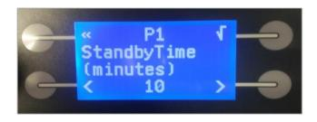
**P1:** standby-time (standstill-time before the machine goes into power saving mode) can be changed
