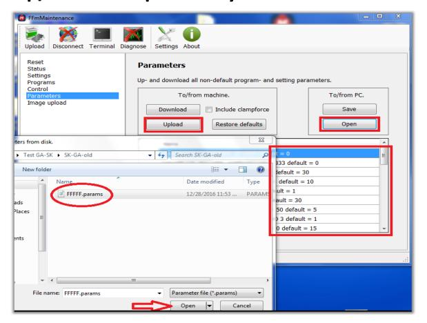
Uploading a textfile with the requested non-defaults to the machine, begins with hitting the "Open"-button to browse to the file. The browser screen opens to be able to locate and select the file. Doubleclicking or hitting "Open" in the browserscreen loads the list with non-defaults into the FFmMaintenance field.
