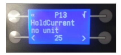
**P13**: The hold current is a certain amount of electrical current through the clamping motor to hold the clampplate in position during shaking. This prevents the clampplate from coming loose during shaking.
