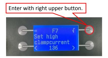
Change the value if necessary (+/-), to check the value place your measure equipment between the plates. Use the CLAMP button to clamp and check the value.(and the upbutton to unclamp.) The plates will move and clamp but there is no shake motion.
