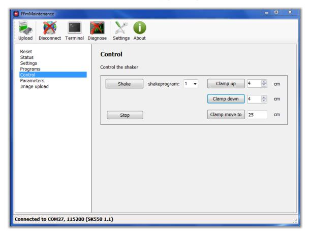
With this functionality, the clampplate can be moved manually over a certain distance ("Clamp Up" and "Clamp Down") or to a certain position ("Clamp move to"), measured from the lowest position upward. Furthermore, the shakeprograms can be chosen, run and stopped manually.
