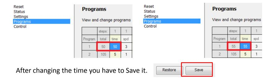
All the "set times" in each time column accumulated, make the total shake time in seconds in the column "total".
