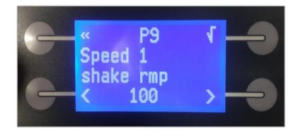
The 6 program times can be changed under **P3-P8** and the 3 shaking speeds can be changed under **P9-P11**
