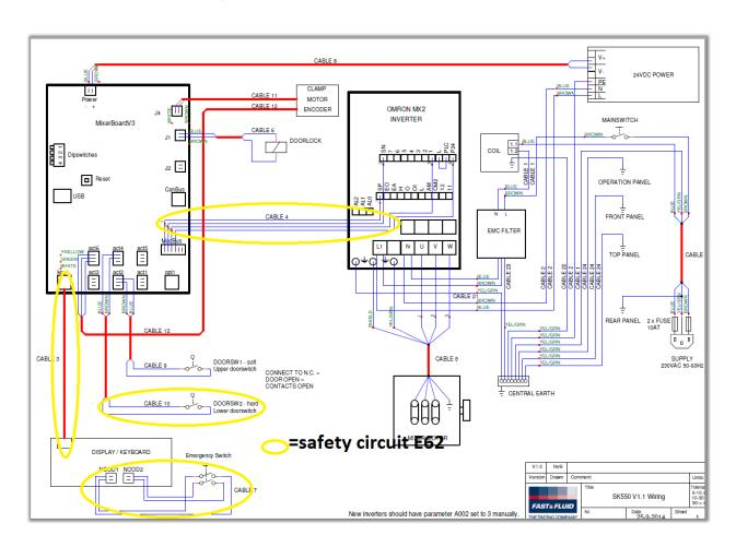
Responsible for errormessages E62 are the components and wiring connections encircled in yellow. The reason is, that machine safety has to be executed in a double fashion. Responsible for errormessage E1 is the upper doorswitch circuit.
