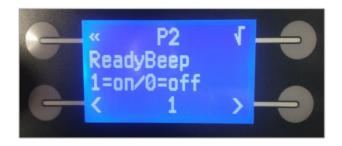
**P2**: The choice can be made to have a beep, indicating that the shake process has finished. The beep sounds at the moment the door is released for opening.
