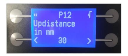
**P12**: The updistance is the distance the clampplate will be raised after shaking.
