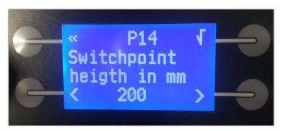
P14: The switchpoint distinguishes between the high clampcurrent being applied (large cans) or the low clampcurrent. (small cans) The value is measured from the bottom table upwards.
