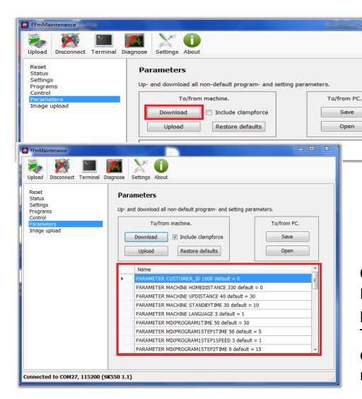
Clicking the "download" button results In listing the non-default program-and parameter settings in the field below. The clampforce can be included or excluded by (un)checking the little box next to the download button
