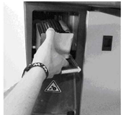
Remove the brush tray by opening the door and pulling down the lever supporting it.
