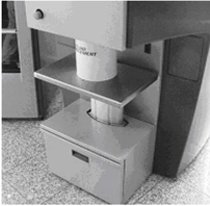
Ensure can opening is under the dispenser nozzle and at its optimal height (automatic stop).
