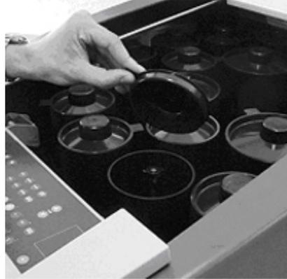
Fill canisters if level is low and update levels in software. Stir colorant beforehand.
