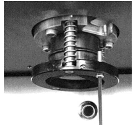
Carefully replace can detection plate and ensure trigger bolt is correctly positioned.
