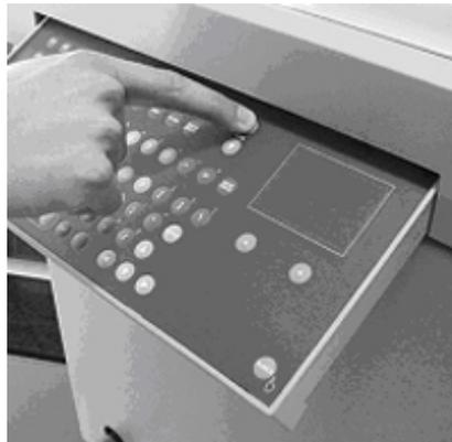
Move the can table upward by pressing the can table switch on the keyboard.
