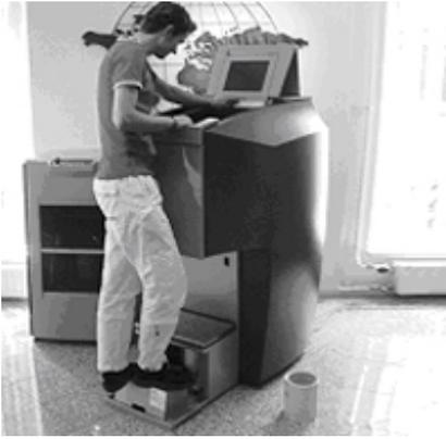
Unfold the step and open the top lid by sliding it all the way back.
