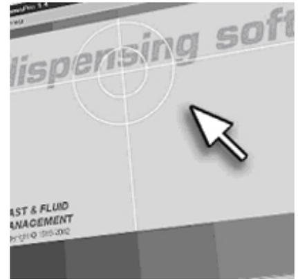
Run software purge program twice to remove air from system.
