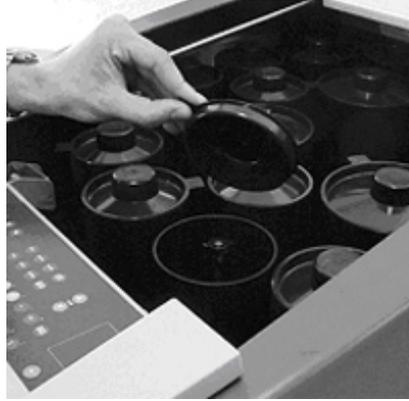
Check canister content and refill if necessary.
