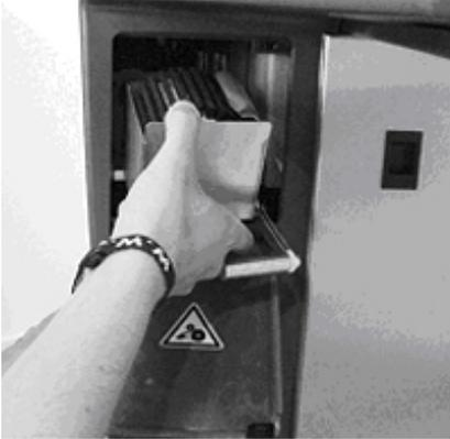
Remove the brush tray and empty the container. Clean the brush with water and refill the container with correct fluid (e.g. water).
