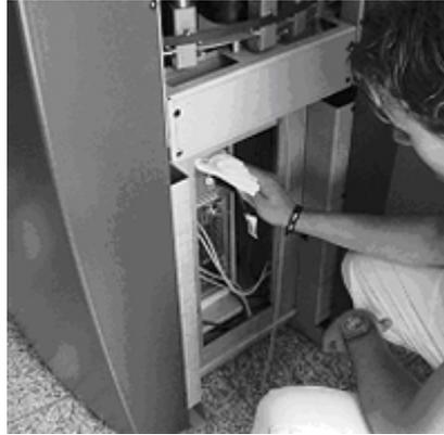
Clean dust from computer cavity and spilt colorant inside machine.
