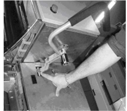
Adjust M4 screws to center punch position under nozzle. Place new (slotted) bottom service panel.
