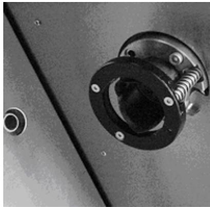
Mount electric punch with three supplied M6 bolts. Take care in positioning the trigger bolt.
