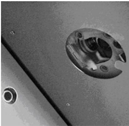
Three nuts for mounting the electric punch are located around the dispense nozzle.
