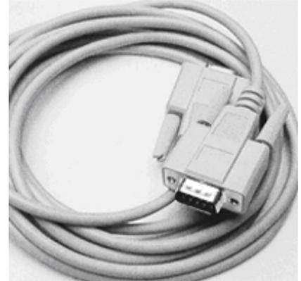
Connect dispenser connector to COM1 (default) and mouse, keyboard and other appliances to designated computer ports.
