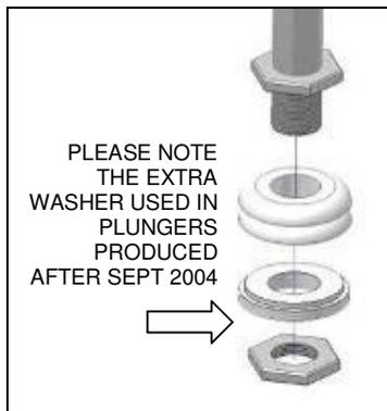
**(2)** Remove the new piston from retainer and fit to the shaft curved end face up (see picture). Replace the front nut using a small drop of Loctite 262 on thread. Tighten the nut only until the piston can no longer be rotated by hand.
