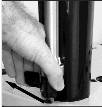
Release the valve lever slowly and the drop will withdraw into the nozzle
