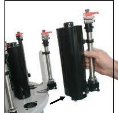
Remove canister from turntable and drain colorant into a clean container
