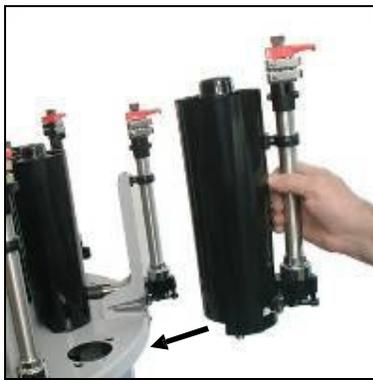
Reassemble and refit canister to turntable
