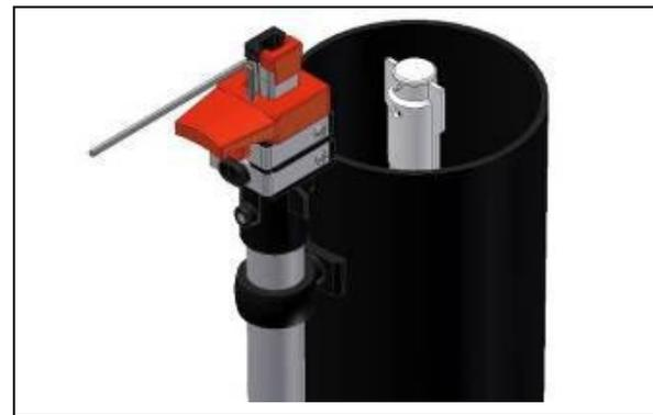
(4) To calibrate the inner (red) plunger, refit the inner (red) gauge and plunger removed in step (1). Set the inner (red) gauge to zero.
