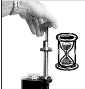
Continue to hold this for a few seconds to ensure the pump is correctly filled with colorant.
