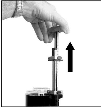
Without operating the valve lever lift the pump handle to its maximum travel (this draws the colorant into the canister)
