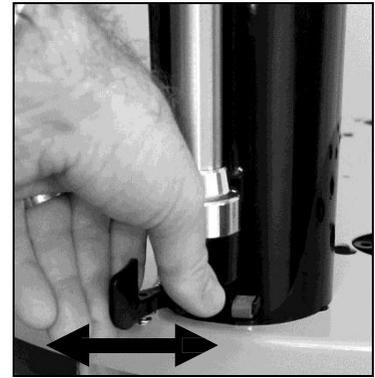
Open and close each pump valve 5 times
