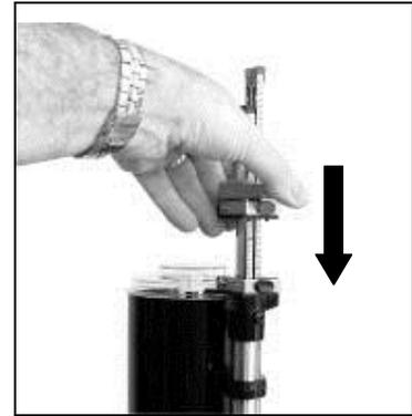
Discharge the colorant back into the canister by depressing the pump handle fully. Repeat this process 30 times.
