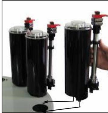
**(2)** Fit the canister screws into the outer ring of keyhole slots on the turntable. Push firmly into position.
