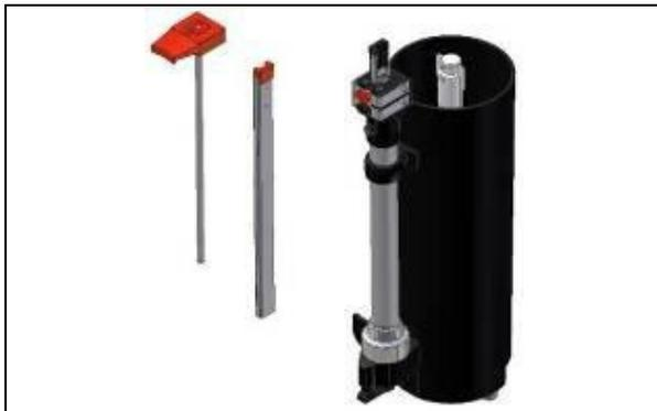
(1) To calibrate the outer plunger, remove the inner (red) gauge and inner (red) plunger and set the outer (black) gauge to the zero position.
