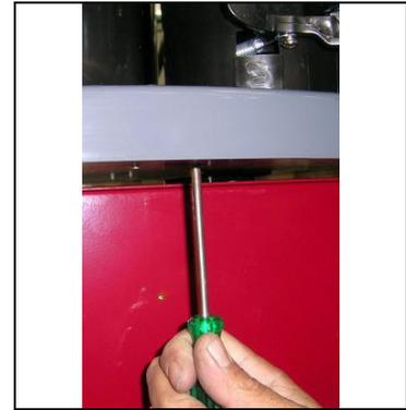
**(3)** Locate the 2 guide holes directly below each canister and fasten the screws (already located in canister) with a Philips (No. 2) screwdriver.
