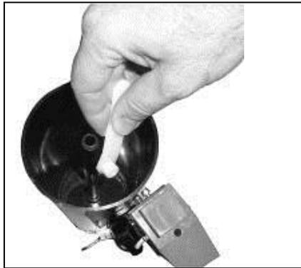
If required, tighten or replace valve insert sleeve (with the wrench supplied). Take care not to over tighten or sleeve with crack.
