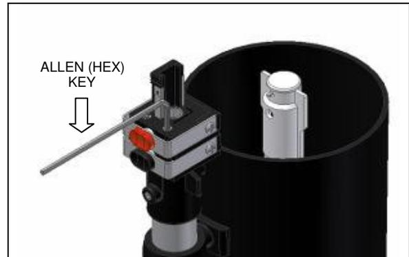
(2) Using the Allen key, undo both calibration grubscrews until free movement can be felt between the outer (black) plunger handle and the outer (black) gauge knob.
