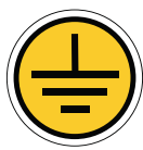
Central earthing point
